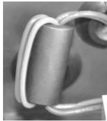
Figure 3-2: Ferrite core and battery supply wiring
