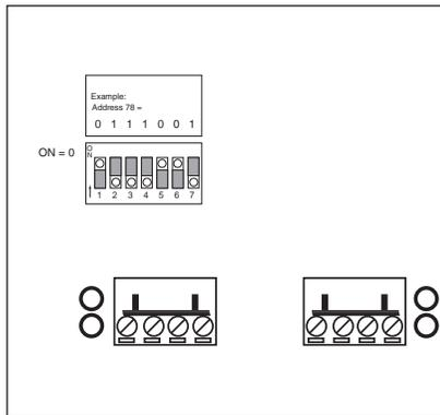
Fig 4 Terminal blocks fitted and address 78 set
