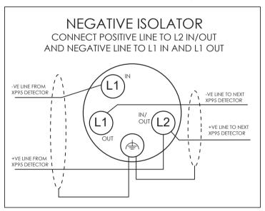
The earth terminal provided is for continuity of screen. Connection to this terminal is not required for operation of the base or isolator connected to it.
